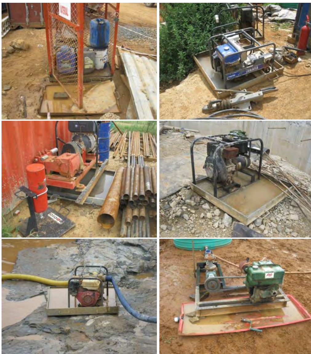
Figure 17: Rain-filled drip trays
