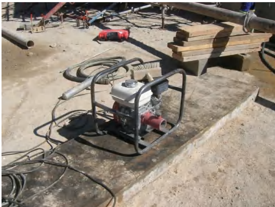
Figure 19: Drip tray required
