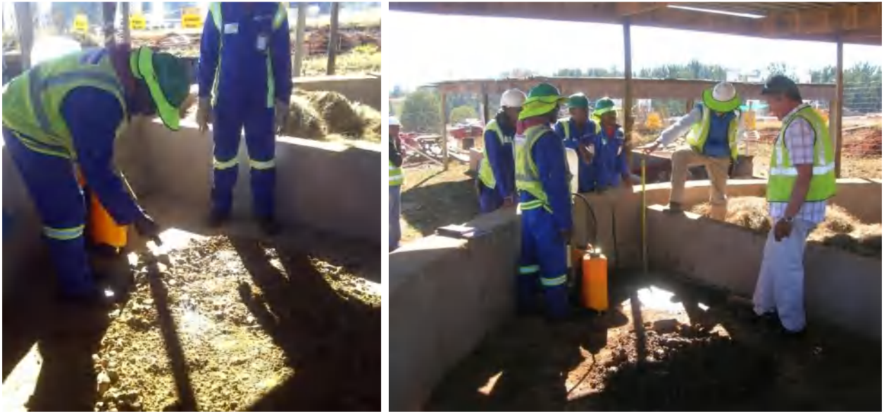
Figure 4: Test trial of substance “Oilcap” (hydrocarbon encapsulator)
