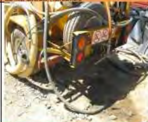
Fig. 6: Lack of proper bunding under parked diesel bowser at left bank.
