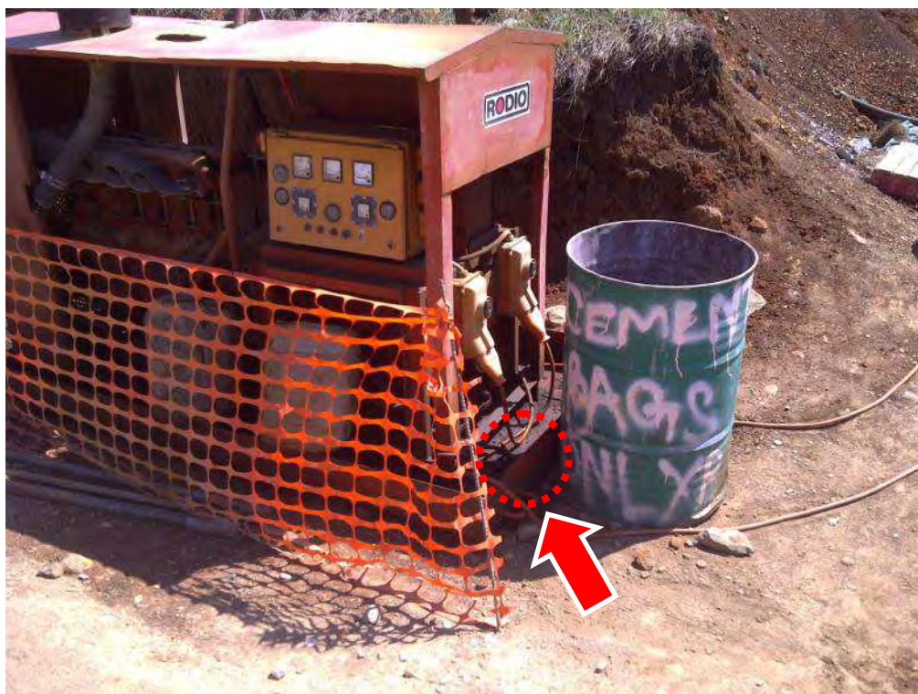
Figure 18: Leaking secondary container
