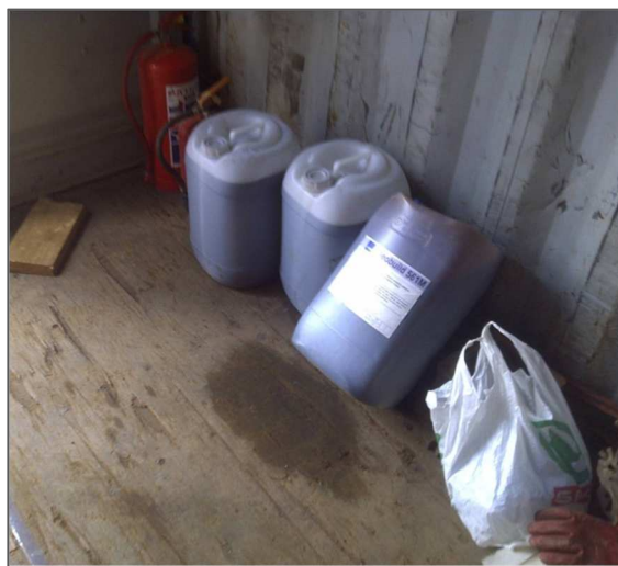
Figure 13: Inadequate storage of hazardous material – area not bunded
