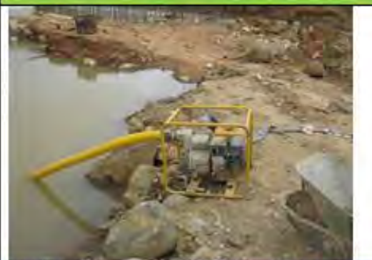
Fig. 21: On 05 December 2012 (date of last weekly inspection), drip trays were missing from under diesel powered equipment in the container at the workshop, RCC trial area and Spring Grove gauging weir (above).
