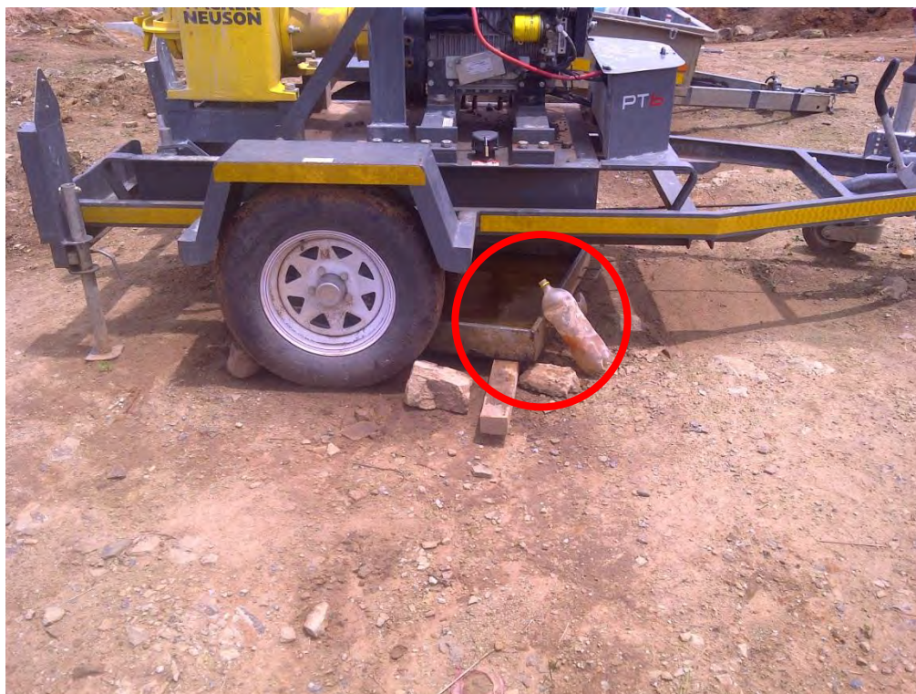
Figure 10: Overflowing drip tray and improper storage of container with hazardous material
